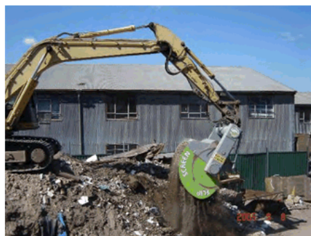
In use, sorting waste material from earth material.
