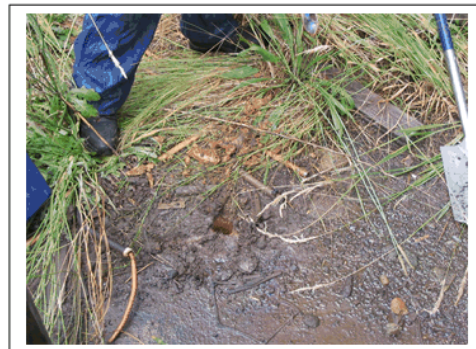
Plate 25. Hydrocarbon Contaminated Soil below the Transformer
