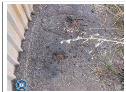
Plate 25. Hydrocarbon Contaminated Soil below the Transformer
