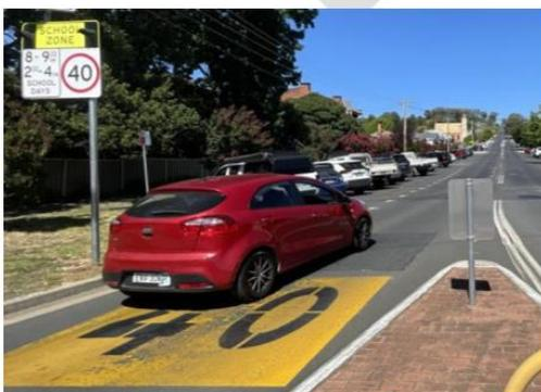
Figure 3-19 40km/h speed zone and dragon's teeth marking (Snowy Valleys School, Capper Street)
