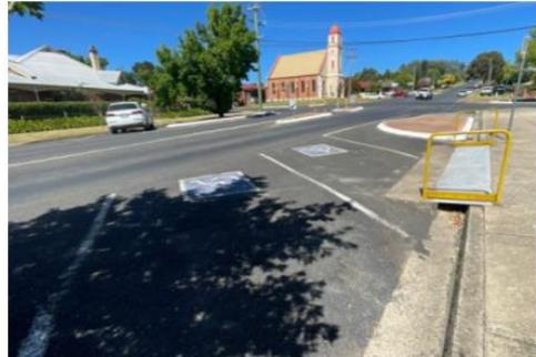
Figure 4-8 Example of Accessible Angle Parking (AS2890.5:2020)
