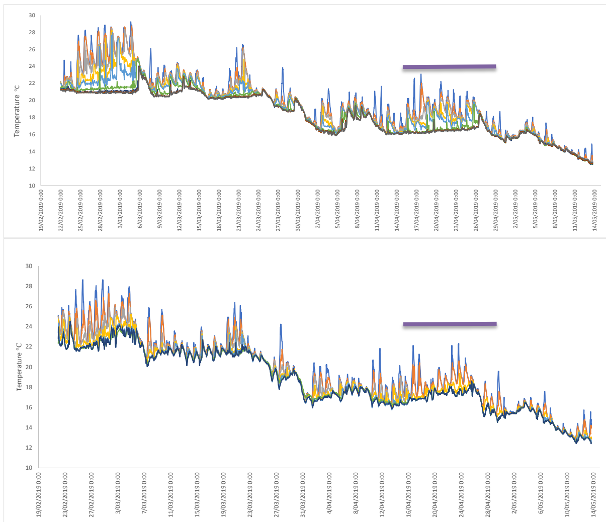
Figure 7. Thermal stratification measured with a thermistor chain at the Outlet site (top) and Pontoon site (bottom) from 1 March 2019 to 14 May 2019. Purple line indicates the period of Dolichospermum and Microcystis growth and bloom.
