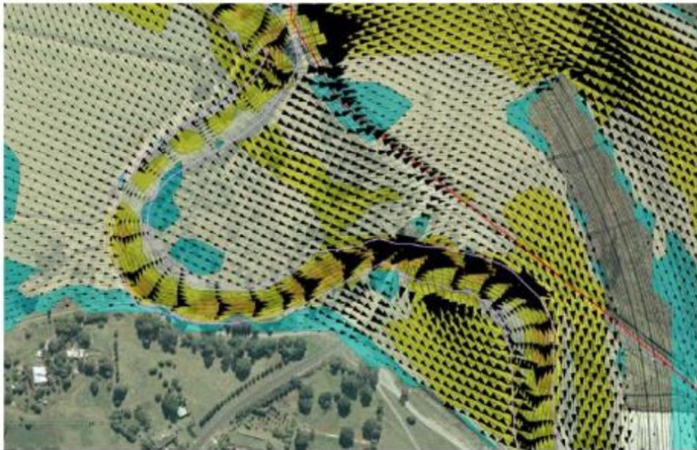
Figure 12 1D/2D Hydraulic Model results showing flow patterns
