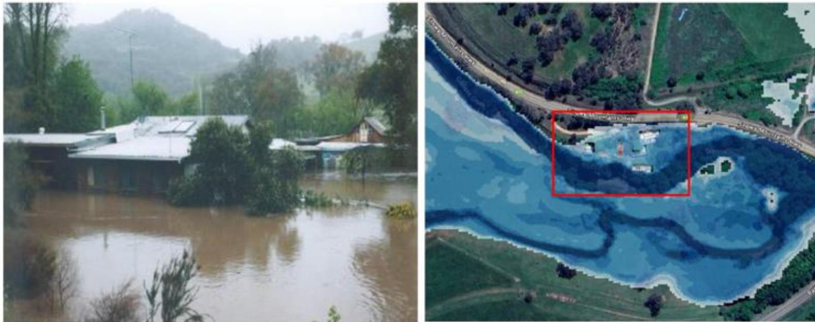
Observed (left) vs Modelled (right) Flood behaviour at Willow Bend
